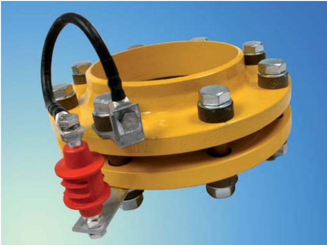
ATEX and IECEx-certified isolating spark gap with a low sparkover voltage for lightning equipotential bonding according to IEC 62305.
