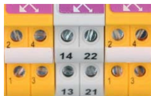
Floating remote signalling contact DRC MCM XT: break contact (21/22) make contact (13/14) DRC SCM XT: break contact (21/22)
