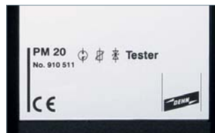
The sparkover performance of gas discharge tubes, varistors and Zener diodes can be tested.
