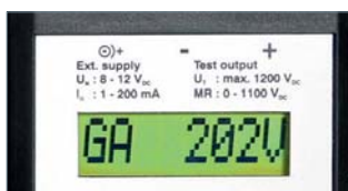
Indication of the measured spark-over voltage.
