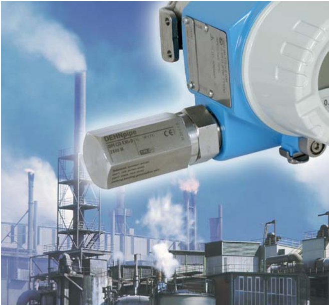
Surge arrester for outdoor use to be screwed onto two-wire field devices. Stainless steel, installation with cable gland up to IP 67.
