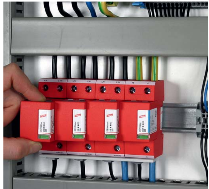
For protecting low-voltage consumer's installations against surges and even direct lightning strikes. For installation in conformity with the lightning protection zone concept at the boundaries from 0_A - 1 (3+1 circuits).
