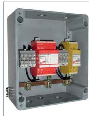
Prewired unit (ITAK) for cathodic corrosion protection consisting of an arrester in a metal enclosure which protects the protective circuit and voltage measuring circuit. Ordering designation: ITAK, serial No. 4305.
