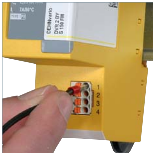
Direct plug-in technology ensures easy conductor connection without tools.
