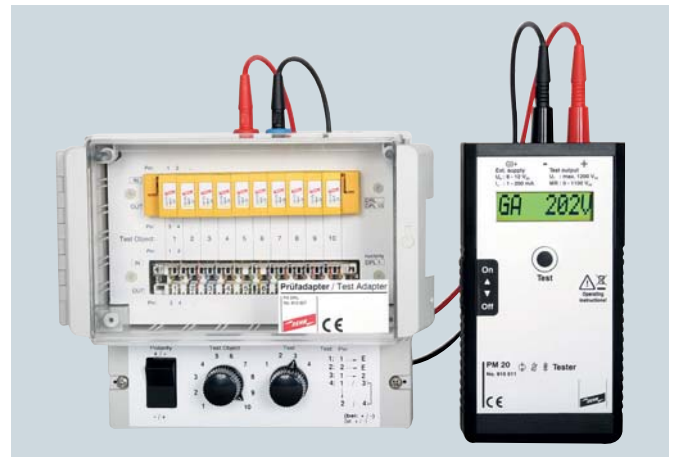
For testing the sparkover voltage of surge arresters. The specimen is connected via the included test leads or special test adapters.
