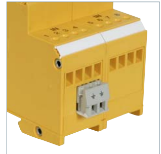
Separate earth connection on the unprotected side of the device. The second slot of the double terminal is intended for connecting the terminal equipment to the equipotential bonding.
